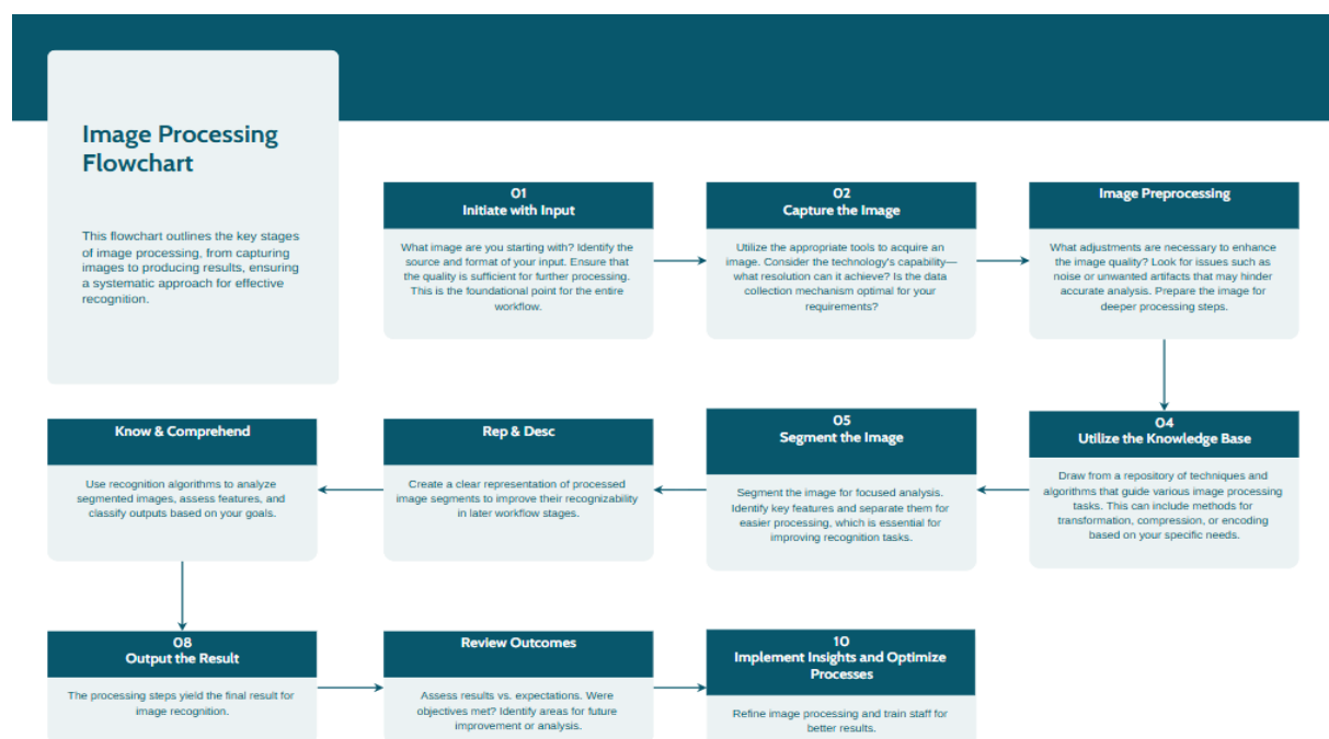
Figure 1: A schematic diagram of the process of image processing (Refer: IMGFLW.com)
